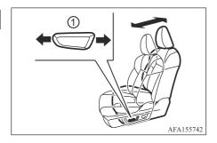
Move forward or backward the adjusting switch ① to the desired position.
