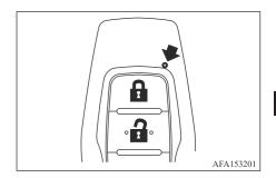
The light blinks only when you push any button on the transmitter. The light illumination only signifies that the transmitter has transmitted a signal. You may look and/or listen to verify that the vehicle has performed the intended operation. If the light does not blink, your battery may be too weak to communicate to the vehicle. If this occurs, the battery may need to be replaced.
