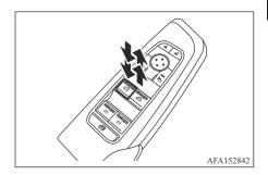
The automatic operation is available for the switch that has an 🖪 mark on its surface.
