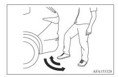
The kick motion sensor (a), located on the back of the rear bumper, enables you to open or close the tailgate in hands-free.
