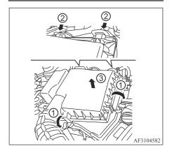
To remove the filter, release the lock pins ①, remove the stoppers from their fittings by sliding the air cleaner filter cover ② and pull the air cleaner filter cover upward ③.
