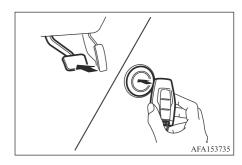
If the battery of the transmitter is discharged, or environmental conditions interfere with the transmitter operation, start the Plug-in Hybrid EV system according to the following procedure:
